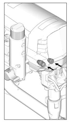
5. Replace plug from step 3 with fitting included with hose reel kit. Torque to 40-50 ft./lbs.
