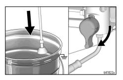
Hold a metal part of the spray gun firmly to a grounded metal pail. Point spray gun into pail. Disengage the trigger lock and trigger the spray gun to relieve pressure.
